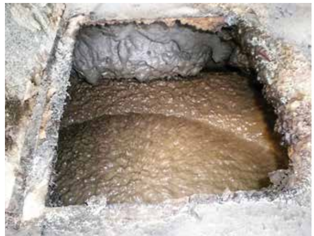
Unstable flow pattern inside the constant headbox
